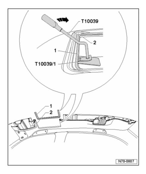
Using the release lever T10039, disconnect the frame in - direction of the arrow from the headliner, the whole way around.
