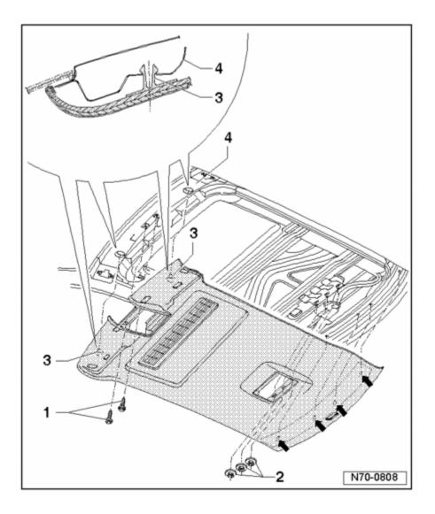
Adjust the front seatbacks as low as possible and remove the headliner from the vehicle through the rear door with the help of a second technician.
