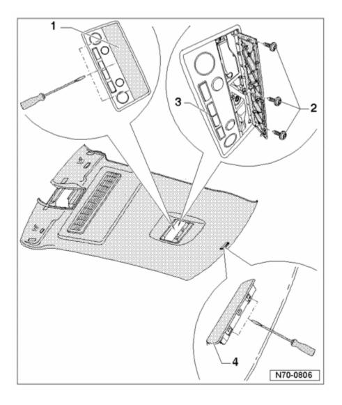
$^-$  Push the wedge T10039/1 between frame -  $\bf 1$  - and headliner -  $\bf 2$  - .
