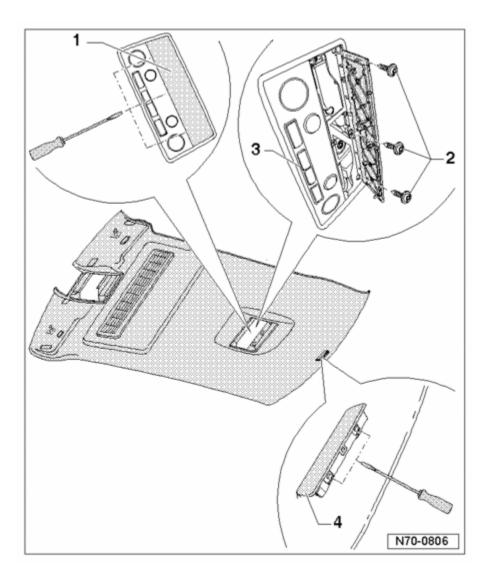
Using a small screwdriver, release the locking tabs from the parking assist system warning buzzer - 4 - and disconnect the wiring harnesses.
