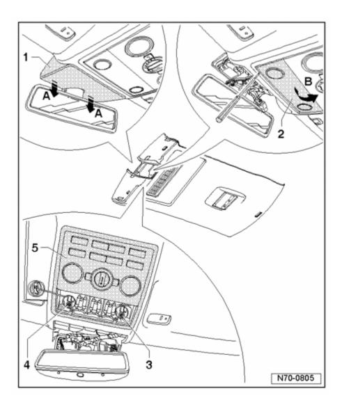
Remove the front illumination and control unit - 5 - from the headliner and disconnect the wiring harnesses.
